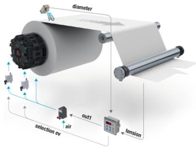
Combined regulation in torque with load cells or dancing roller
