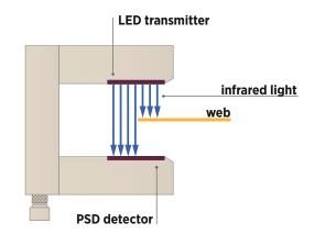
SIR.m-25 is equipped with a PSD detector and infrared LEDs on the opposite side that generate infrared light which is converted by the PSD into electric signals. According to the intensity of the signal received, the microprocessor can identify how much of the sensitive surface of the capsule is covered by the material inserted in the fork and calculate the position of the web edge.
